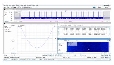
Shown above is a 700 MHz wide chirped signal. A time overview is presented at the top of the display that shows the pulses in the current acquisition. Phase deviation is displayed on the left, showing the characteristic parabolic shape of a frequency chirp. The signal has variations in repetition interval, shown in both the pulse table and the spectrogram on the right.
