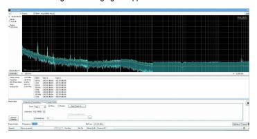
The RSA7100B's intrinsic phase noise of -134 dBc/Hz, at this frequency and across its operating range, provides ample measurement margin for a vast majority of applications.
