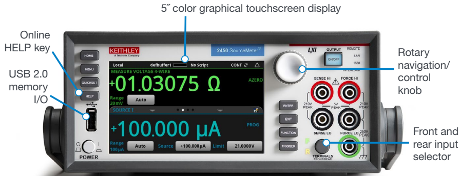
2450 front panel with high-resolution, capacitive touchscreen.
